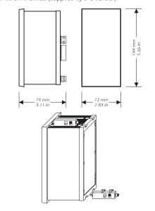
installation with screw brackets; moderate the clamping torque, in order not to damage box and screw brackets.
