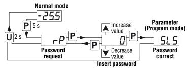
**Note:** If the Password gets lost, just switch OFF and ON the instrument, push  $\bigcirc$  key during the initial test keeping it pressed for 5 s. In this way it is possible to access all the parameters, verify and modify the parameter  $E^{PP}$ .
