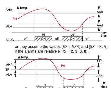
The maximum and minimum temperature alarms can be disabled by setting the related parameters BHB and BLB = oF. The temperature alarms are signalled lighting up the alarm LED ( $\triangle$ ) and, if configured, also with the buzzer
