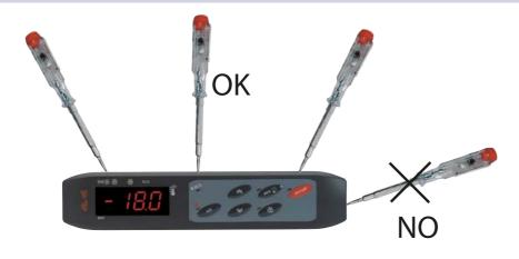
To remove the front operate on the three fastening hooks as indicated in the figure (from above or from below but never from the side)
