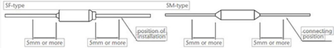
If soldering, take note that the thermal link may function because of excessive solder temperature. To prevent such malfunctions, for example, holding the lead near the case with a tool is effective for allowing the heat to escape and the soldering should be done in short intervals.
