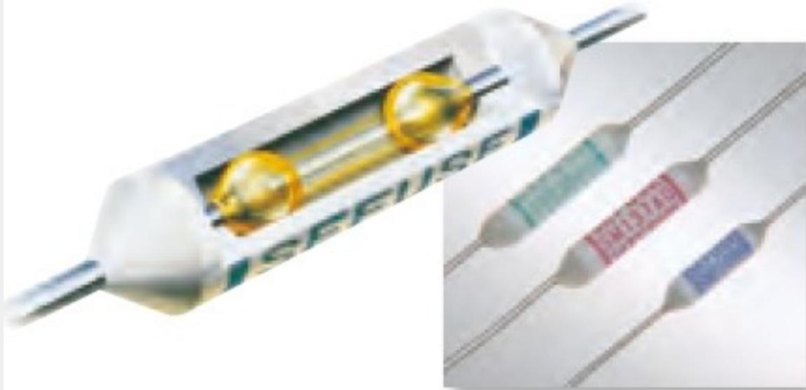
The SM-type uses a fusible alloy inside a ceramic case. As ceramic is an insulator, the SM-type can be fixed directly where temperature detection is required. The SM-type has a rated current of 0.5A to 2.0A (AC) / 3.0A to 7.0A (DC).
