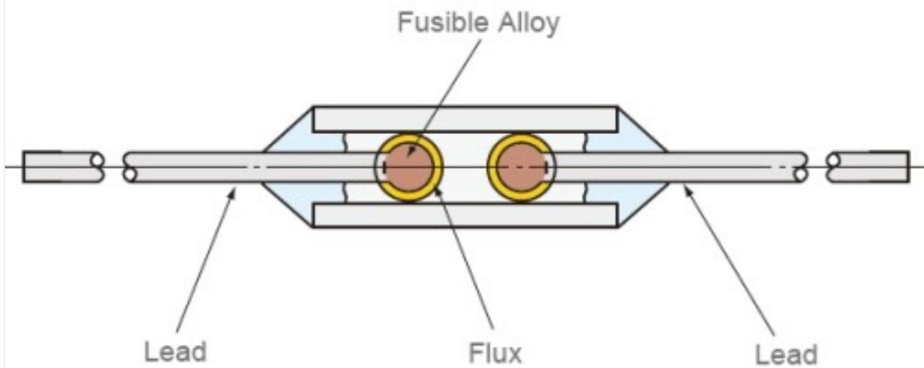
When the ambient temperature rises to the operating temperature of the SM-type, the fusible alloy melts and forms a drop around the end of each lead due to the surface tension and the special flux coating. Without a direct contact between the leads, the electrical circuit is opened.
