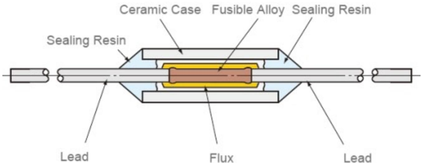
The leads of the SM-type are connected by a fusible alloy thereby allowing the current to flow directly from one lead to the other. The fusible alloy is coated with a special flux.
