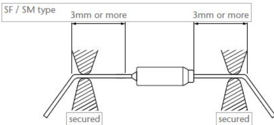
The tensile strength applied to the lead wire should be 49N or less for SF-type and 9.8N or less for SM-types.
