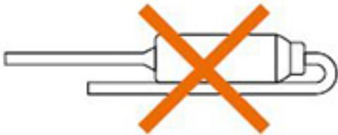
Note that the body of the SF-type is the same in potential as the circuit. Therefore, it must be electrically isolated from other metallic parts.
