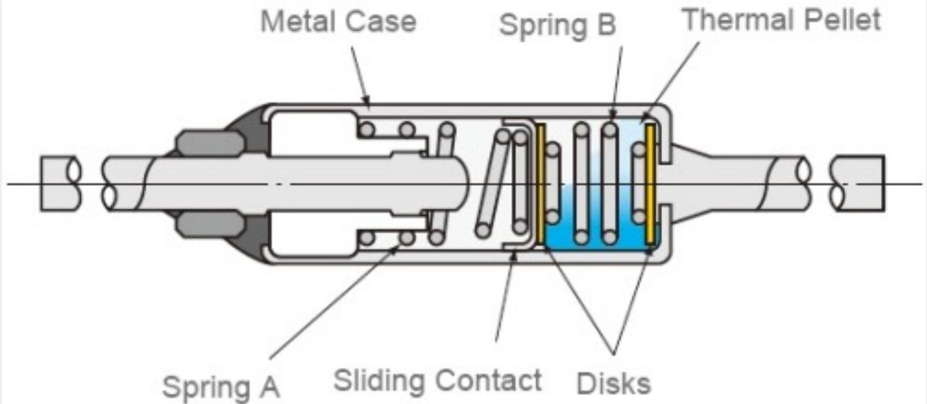
When the ambient temperature rises to the operating temperature of the SF-type, heat is transferred through the metal case and melts the thermal pellet. Springs A and B then stretch and the sliding contact moves away from lead A, thereby opening the electrical circuit.
