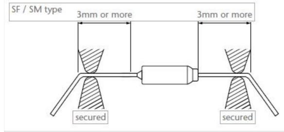
The tensile strength applied to the lead wire should be 49N or less for SF-type and 9.8N or less for SM-types.
