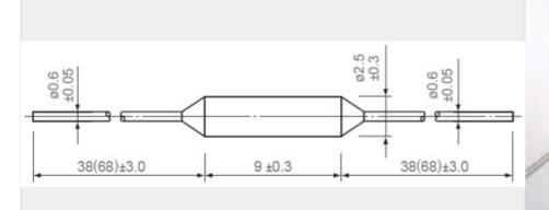
Note: The dimensions for long lead devices are in parentheses.
