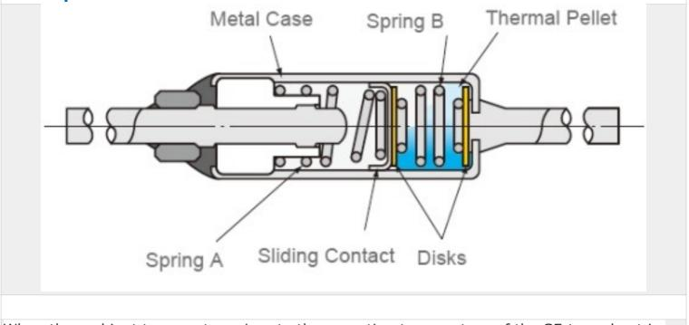
When the ambient temperature rises to the operating temperature of the SF-type, heat is transferred through the metal case and melts the thermal pellet. Springs A and B then stretch and the sliding contact moves away from lead A, thereby opening the electrical circuit.
