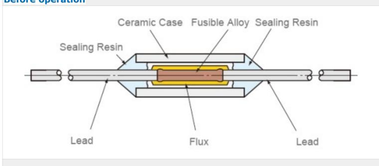
The leads of the SM-type are connected by a fusible alloy thereby allowing the current to flow directly from one lead to the other. The fusible alloy is coated with a special flux.
