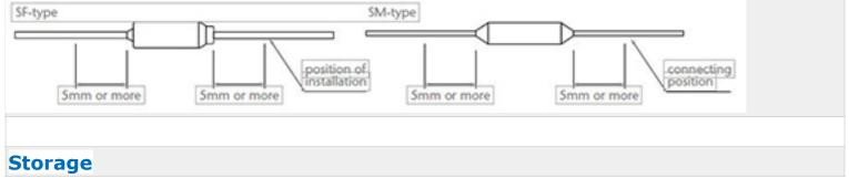
The body and lead A of the SF-type, and the leads of SM092A, SM092B, SM225A, SM225B and SM225G are silver-plated. Therefore, these parts may discolor because of sulfuration, making the markings on the body illegible or negatively affecting the solder-ability of the lead. To avoid this, the thermal link should not be kept around materials (such as cardboard or rubber, etc.) which generate sulfurous acid gas.
