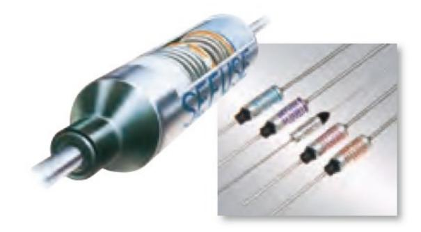
The thermal pellet placed inside the metal case of the SF-type responds to an abnormal temperature situation and triggers the cutoff function. The SF-type features a large rated current of 6A to 15A (AC). Furthermore, the SFH/R series has higher Tm than conventional thermal links, as well as excellent insulation performance at high temperature conditions.
