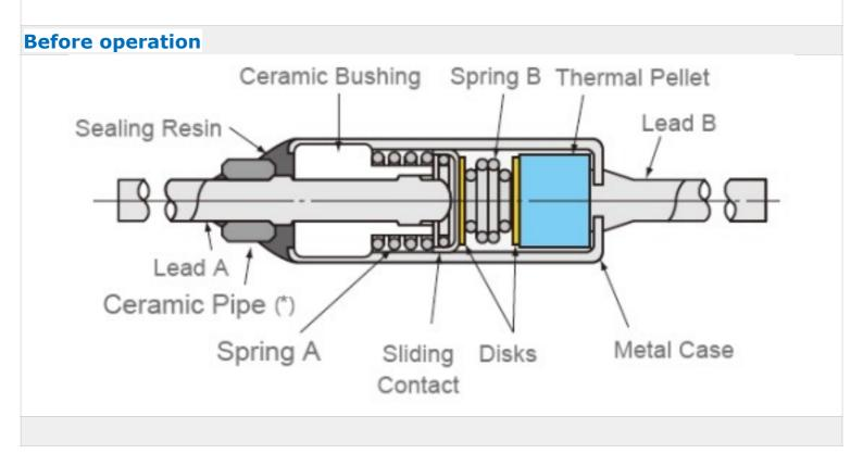
The SF-type contains a sliding contact, springs and a thermal pellet inside a metal case. When spring B is compressed, there is firm contact between lead A and the sliding contact. At normal temperatures, current flows from lead A to the sliding contact and then through the metal case to lead B.
