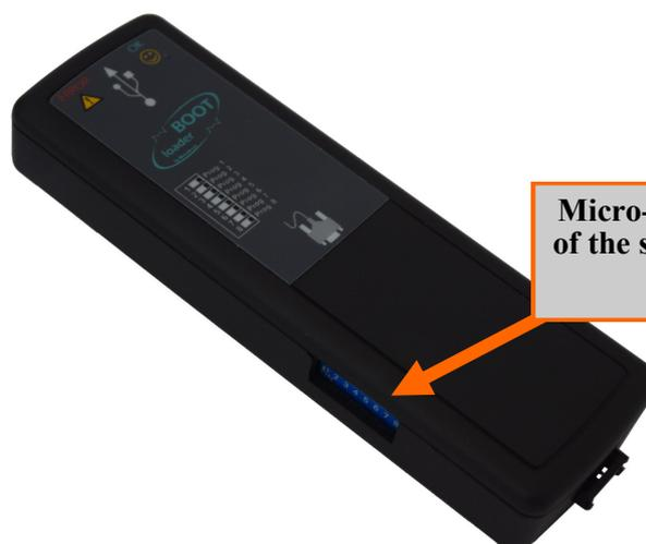
Micro-switches for the selection of the software to be installed on the card
